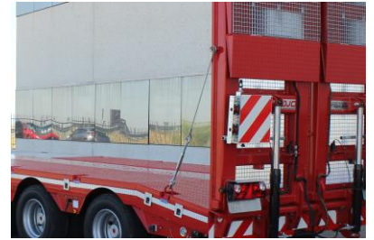
Fig. 4.8 Security cable ramps
